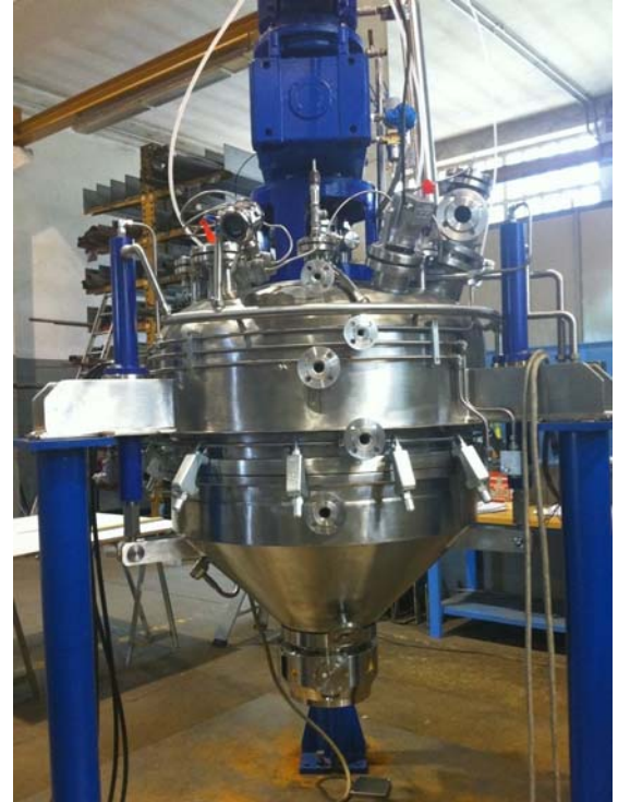
Condry® conical bottom agitated vacuum dryer, left in Titanium Grade 7, right in Hastelloy C 22
