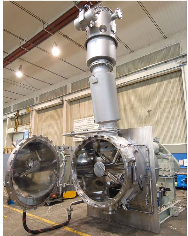
Pharmadry® paddle dryer, left as vacuum dryer, right in pressure proof version
