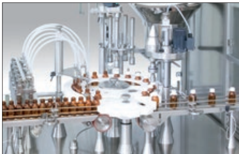
Transport systems by starwheels
