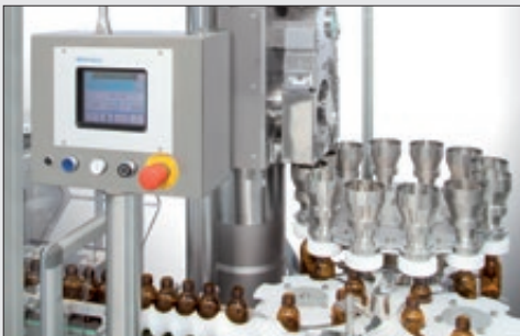
Powder filling station
